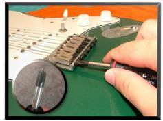
(Example: If the 2nd string is. 011" you would move the 2nd string back .011" from the  $1^{st}$  saddle). Move the 3rd back from the  $2^{nd}$  saddle, using the gauge of the 3rd string as a measurement. The  $4^{th}$  string saddle should be set parallel with the  $2^{nd}$  string saddle. Proceed with the  $5^{th}$  and  $6^{th}$  in the same method used for strings 2, and 3. Each string should resonate naturally at the  $12^{th}$  fret.
