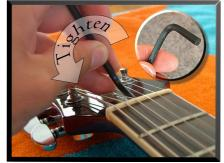
**Setting Your String Height** Players with a light touch can get away with lower action, others need higher action to avoid rattles. Check tuning. Using a ruler, measure distance between bottom of strings and top of the 17th fret. Adjust bridge saddles or if your saddles are preset, the bridge height adjustment screws, to approximately 1,5mm. Experiment with the height until the desired sound and feel is achieved.
